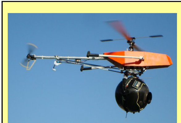
A simplified 4 blades Camera Helicopter. This device is battery operated and can operate for about 10 minutes carrying an 8.5 pound payload, in this case a 35 mm camera. This model is rather pricy at about $17,500 but less ambitious model helicopters can easily be purchased at hobby shops for as little as $50.00.
